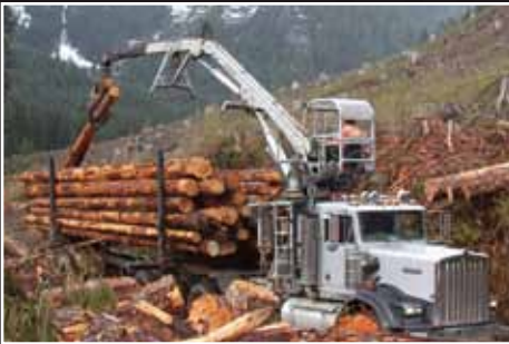
Each site has a self-loading tractor-trailer rig for moving the logs to water.
