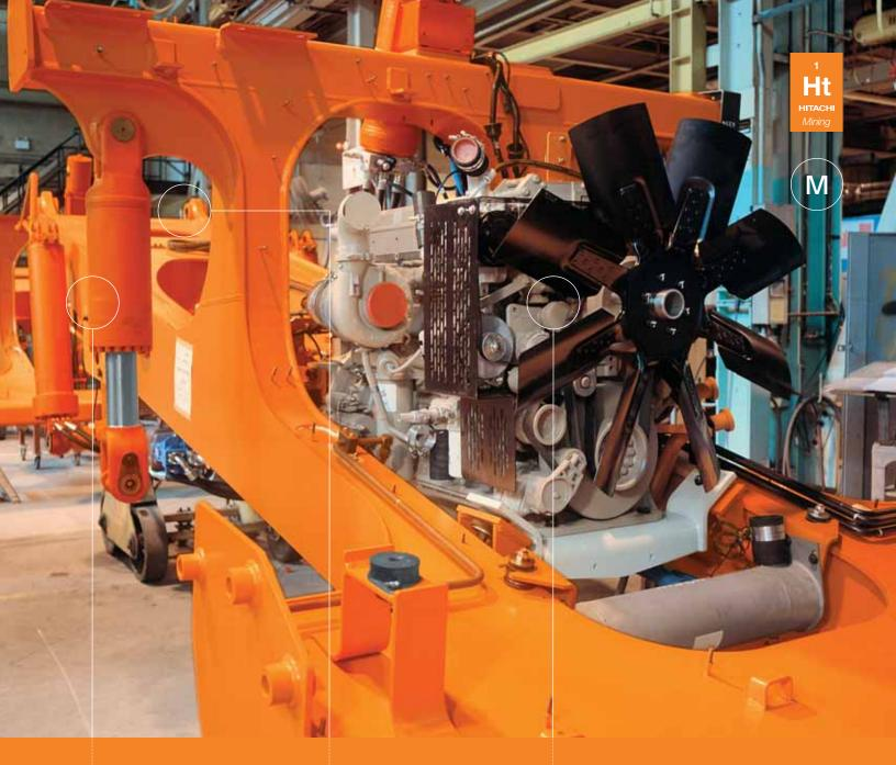
Vertically mounted struts absorb haul road input and minimize frame twisting.
