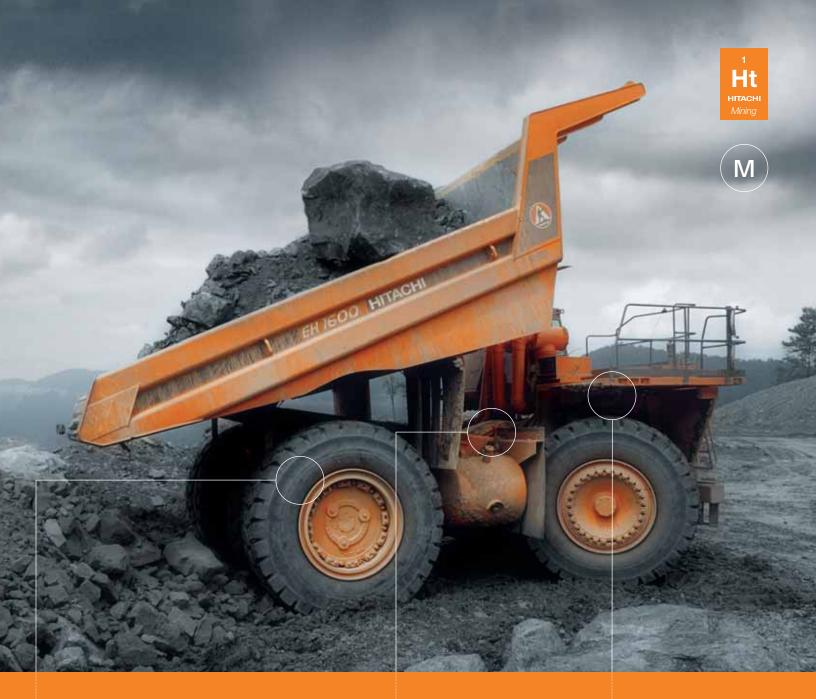
The plug-in design of the rear drive axle delivers outstanding ease of service because it is easy to remove and install. A "high-speed" ratio is optional.
