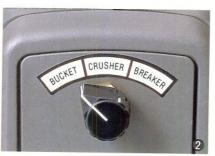
Extra Port that Sets Optimum Flow to Optional Attachment: The extra port is a hydraulic source for setting and delivering the optimum oil flow to optional attachment that is well matched with the front attachment. Attachment Mode Optionally Available: The attachment mode can be selected with the attachment selection switch according to the
