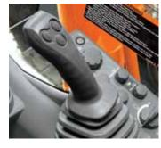
■ The short-throw pilot levers are ergonomically correct for smooth, precise control with less movement and effort. When digging conditions become more demanding, the operator can handle it by simply pressing the power boost button.
