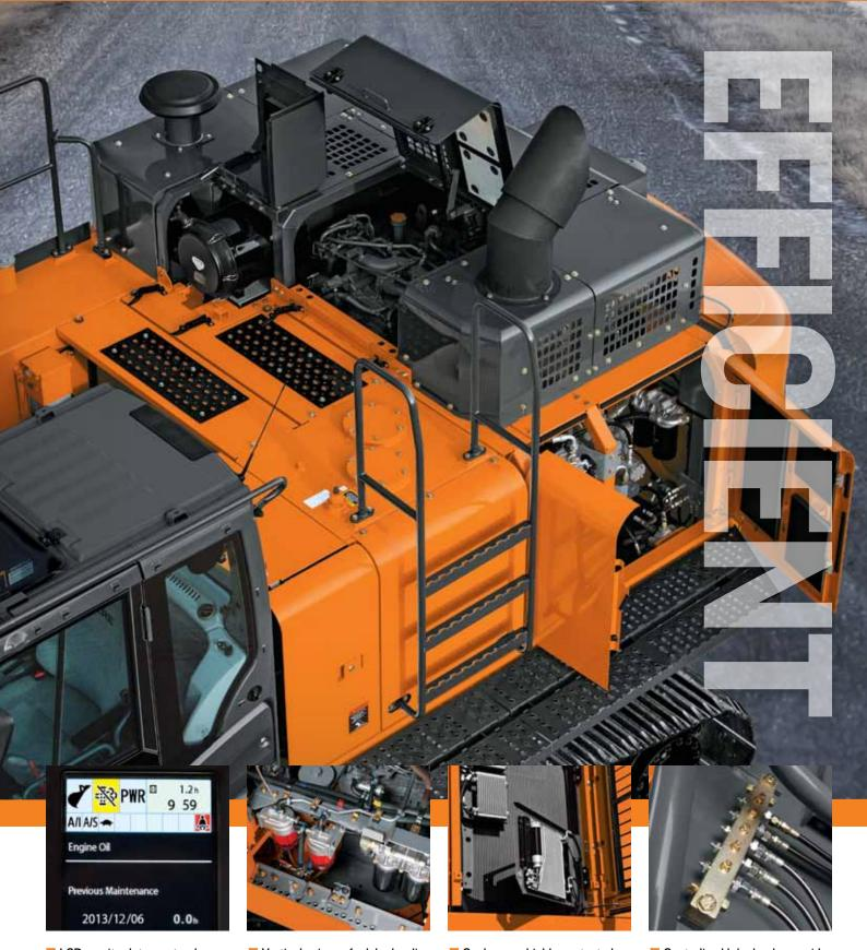
■ LCD monitor lets you track scheduled maintenance and reminders, plus provides diagnostic codes to assist in troubleshooting. ZXLink™ also provides early warning and remote diagnostics.
