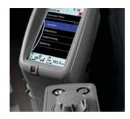
■ Multi-language LCD monitor and rotary dial provide a wide variety of information and control. Simply dial and tap to select work modes, monitor maintenance intervals, check diagnostic codes, set cab temperature, tune radio, make simple attachment hydraulic adjustments and much more.
