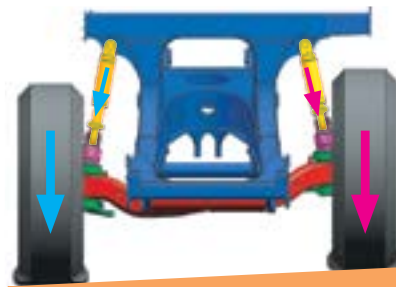
DRIVER SIDE STRUT IN COMPRESSION, OTHER STRUT IN EXTENSION
