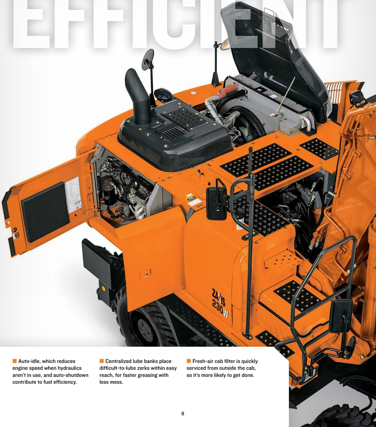
■ Auto-idle, which reduces engine speed when hydraulics aren't in use, and auto-shutdown contribute to fuel efficiency.
