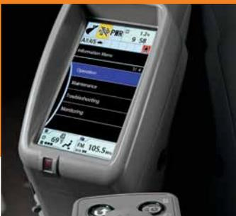
■ Multilanguage LCD monitor with integrated radio and HVAC provides easy access to maintenance alerts, diagnostics, rearview camera visual display and more.
