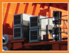
■ Retarding grid boxes are Hitachi built. Each is equipped with an inverter-controlled variable-speed cooling fan.
