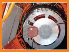
■ AC wheel motors are oilcooled with coolers located in the rear axle box.
