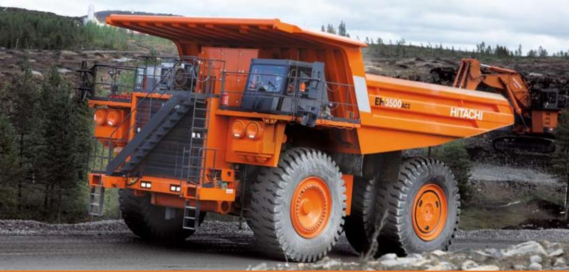
TARGET GMOW: 681,200 LB (309 000 KG) RATED POWER: 2,000 HP (1491 KW)
