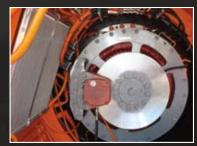
■ AC wheel motors are oilcooled with coolers located in the rear axle box.
