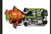
■ Double-path tandem-planetary design provides longer lubricant life, lower operating temperatures, and improved component life.
