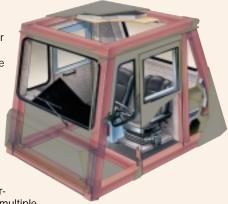
layered floor mat act to absorb sound and control interior temperature. A properly maintained cab from Euclid, tested with doors and windows closed per work cycle procedures in SAE J1166, results in an operator sound exposure  $L_{\rm eq}$  (Equivalent Sound Level) of 81 dB(A). A three-point rubber iso-mount arrangement to the deck surface minimizes vibration to the operator compartment.
