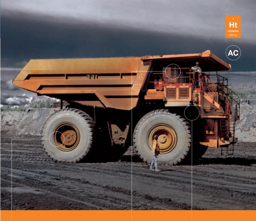
AC traction motors have a high power-to-weight ratio. Brushless design eliminates brush failure and replacement. Dynamic retard minimizes hydraulic brake wear and tear. Dynamic retard is so effective that the hauler can be slowed to .5 mph (0.8 km/h) without the operator ever touching the brakes.
