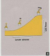
**Te-P Control:** The E-P control system computer regulates the engine output and pump delivery flow to suit job requirements. The electronic engine speedsensing control system controls the pump by detecting changes in engine speed with each new load. This permits maximum use of engine horsepower. For each job, you can select the optimum operation mode which best suits your needs: SP mode for heavy-duty, P mode for general, E mode for energy-saving and L mode for light-duty operation.
