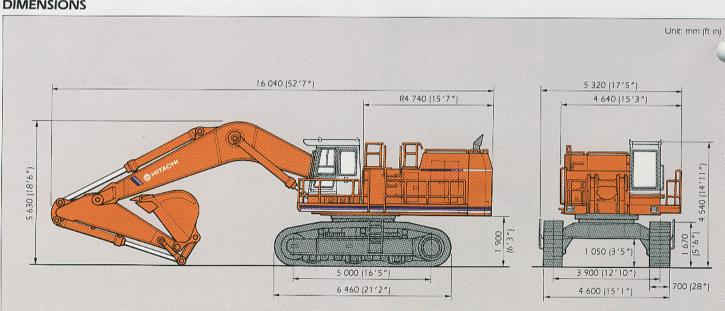
Note: Applicable for 4.6 m³ (6.0 cu yd: PCSA heaped) bucket, 9.1 m (2911 f) boom, 3.4 m (11 '2") arm and 700 mm (28") shoe.
