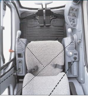
The work modes, power modes, air conditioning controls, and dial-type engine speed control are all located beside the operator.
