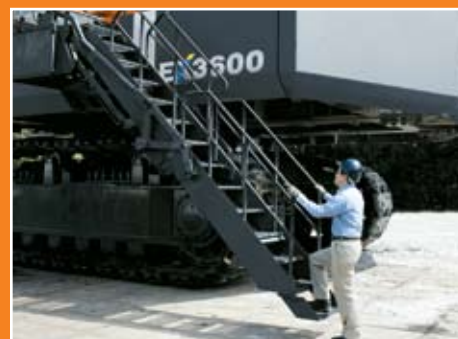
■ Steps fold hydraulically on EX2500-6 and larger models — optional on EX1900-6.
