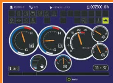
■ 10.5-inch color LCD monitor displays operating and sensor-fault information.
