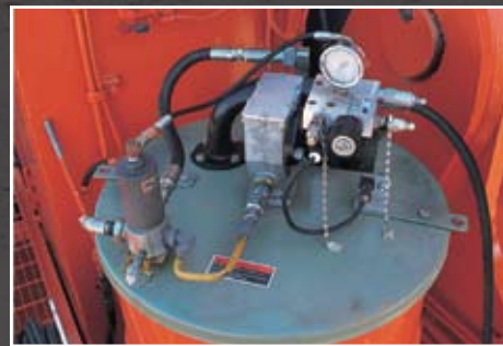
■ AUTO-LUBRICATION: Automatically lubricates all bucket and front-attachment pins and swing bearing.
