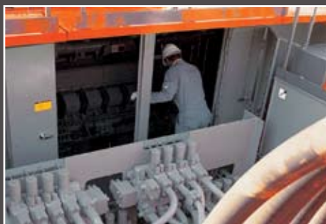
■ WIDE-ACCESS SERVICE DOORS: For easy access to all components and machine servicing areas.
