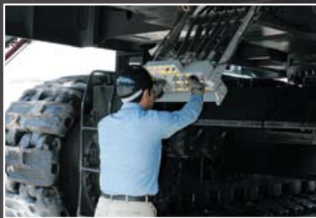
■ FAST-FILL SYSTEM: Ground-level access for fast, easy, and clean replacement of machine fluids, including fuel, coolant, and lubricants.
