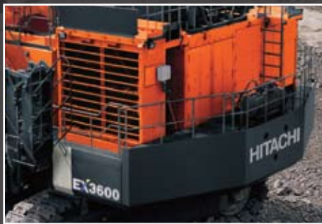
■ COUNTERWEIGHT WALKWAY: Allows easy access to engine, pumps, and radiator for service and inspections.
