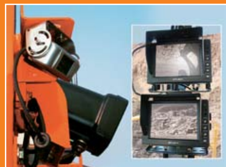
■ With remote cameras, the operator has virtually no blind spot.
