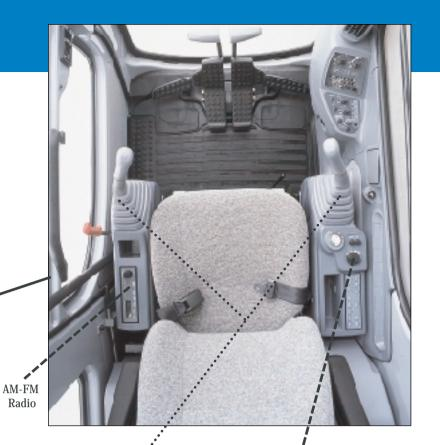
The hand control levers can be raised or lowered to match the operator's build, and the controls can either glide forward or back with the seat or remain fixed while the seat moves.
