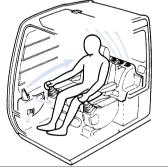
Air conditioning and a "Hot and Cool" box are standard on the EX200. The large capacity unit features front and rear rotatable louvers. Automotivetype controls blend hot and cold air to provide the perfect temperature.
