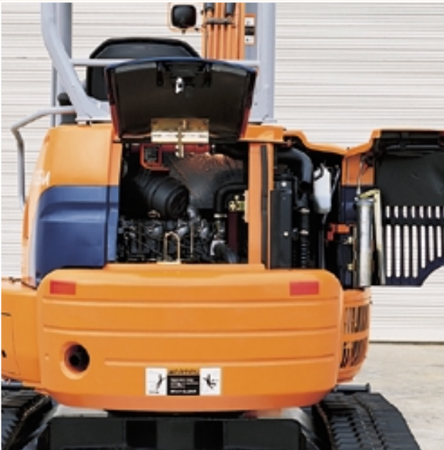
Engine cover opens wide for easy maintenance
