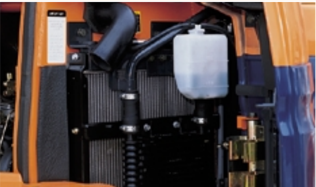
Aluminum-finned radiator and oil cooler for high resistance to corrosion
