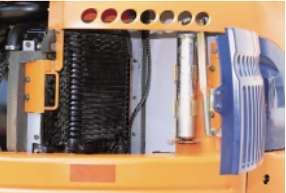
Aluminum-finned radiator and oil cooler for high resistance to corrosion
