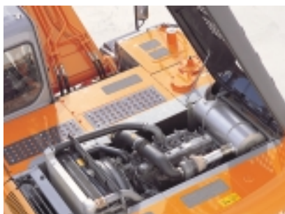
A low-noise muffler and the Isuzu Tier II emissions control engine ensure a quieter, more environmentally friendly excavator. Plastic parts are labeled for easy recycling. Wiring is lead-free.
