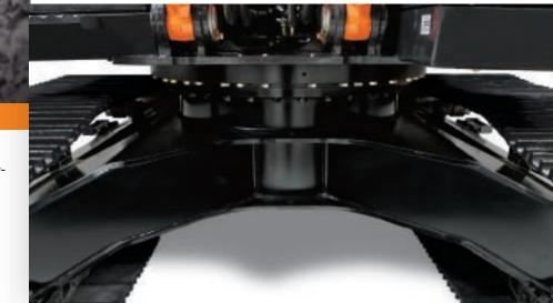
Thick-plate single-sheet mainframe, box-section track frames, and industryexclusive double-seal swing bearing deliver rock-solid durability.
