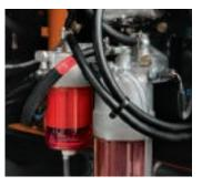
Vertical spin-on fuel- and engine-oil filters are positioned in the right rear compartment for simplified ground-level servicing.
