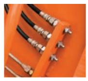
Centralized lube banks places zerks within easy reach to make greasing less messy and time-consuming.
