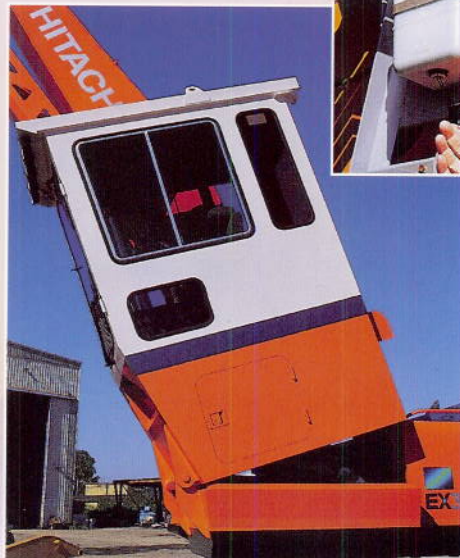
Above: Optional rear entry cab/riser with standard hydraulic tilt features safety interlocks, hydraulic raise/tilt powered by electronic pump
