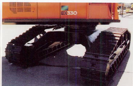
High and Wide undercarriage is designed to handle tough forestry terrain
