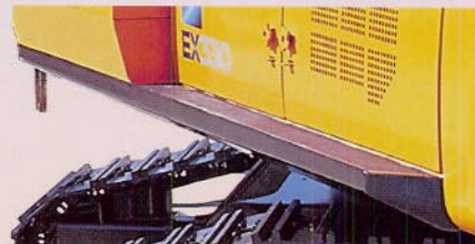
Standard 10-inch (254 mm) wide catwalks are mounted for optimum machine access and protection along both sides
