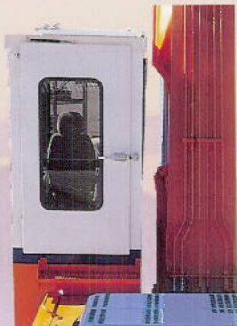
Rear Entry Cab provides safer access and larger, more comfortable work station than conventional cab
