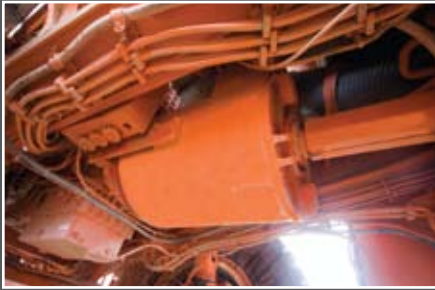
■ IGBT ALTERNATOR: Assembled inside the liquid-cooled inverter cabinet for longer life.
