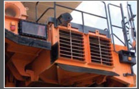
■ 14- TO 20-GRID ELEMENTS: Efficient air-cooled grid box for superb retarding capabilities.
