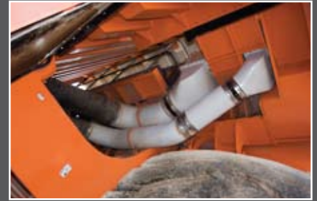
■ AIR TO ALL COMPONENTS: Alternator and wheel motors receive ducted air from their own separate blower motors and fans.
