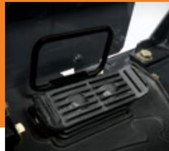
■ Swing boom and foldable travel pedals on the ZX26U-5 and ZX30U-5 are positioned where they're easy to operate, yet allow plenty of foot room.
